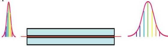
Fig.2. Pulse broadening due to chromatic dispersion
