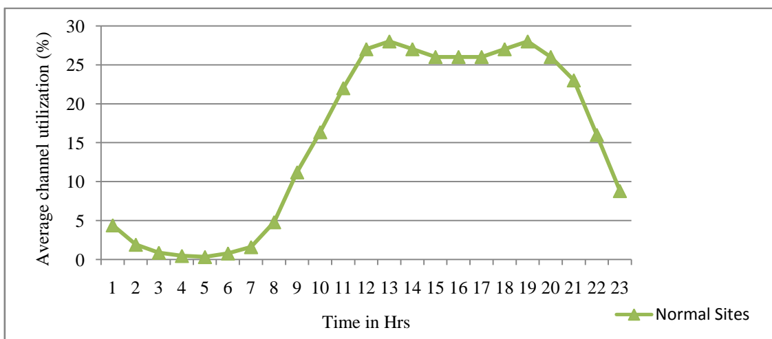
Fig. 3 Average channel utilization characteristics of normal sites before optimization
