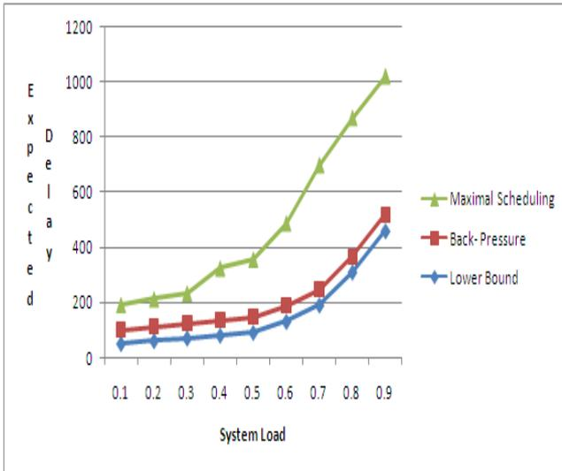
Fig. 6: shows simulation results for tree topology
