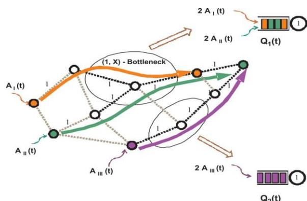
Fig. 1 – Multihop wireless network with bottlenecks (excerpt from [1])
