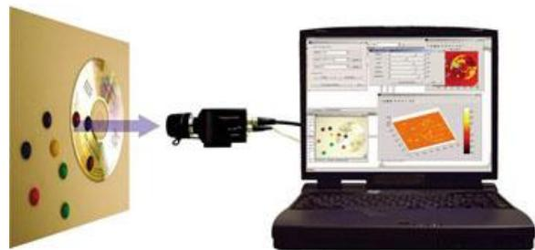
Figure 1: The Scientific Camera captured images are acquired using Image Acquisition Toolbox and analyzed using Image Processing Toolbox
