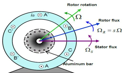
Fig.1: Squirrel cage rotor AC induction motor cutaway view
