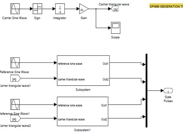
Fig..8: Carrier wave and reference wave
