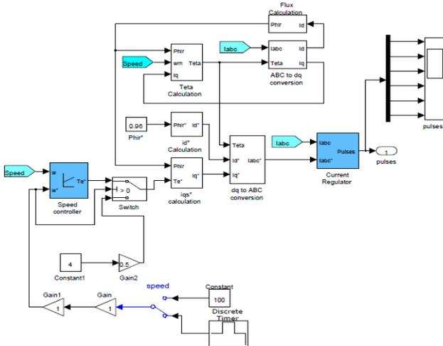
Fig.14. Simulink model for vector controller
