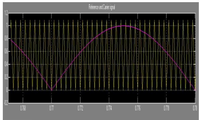
Fig.10: carrier and reference waves
