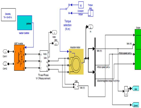
Fig.13: vector controlled inverter circuit
