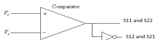
Fig..3: Bipolar PWM generator
