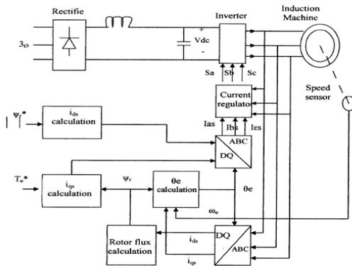
Fig.4: Block diagram of an indirect vector-oriented control system for an induction motor
