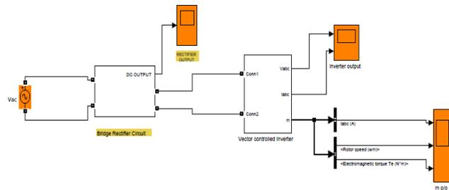
Fig. 5: simulink module for ac/dc/ac converter for closed loop operation of IM
