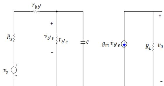
Fig.3. Simplified High-Frequency Equivalent Circuit
