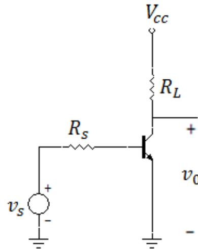
Fig.1. Common-Emitter Amplifier
