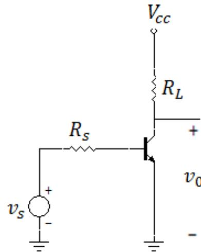
Fig.1. Common-Emitter Amplifier
