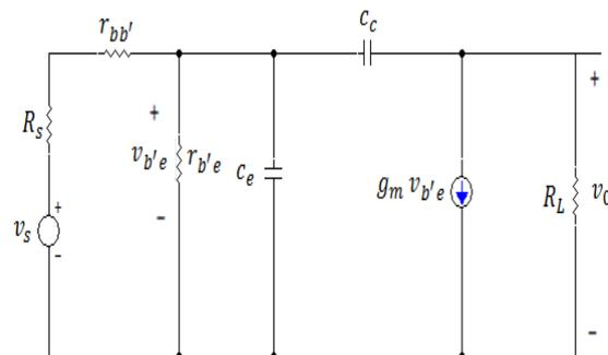
Fig.2. High-Frequency Equivalent Circuit
