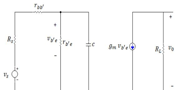
Fig.3. Simplified High-Frequency Equivalent Circuit
