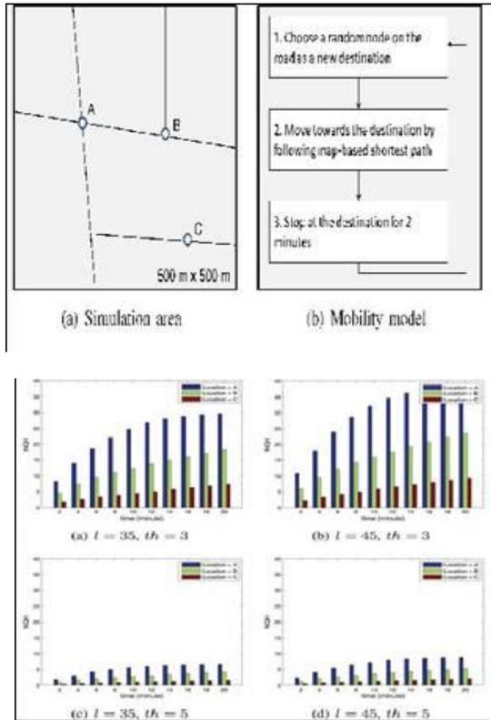
Fig.2. Simulation area and mobility model under consideration
