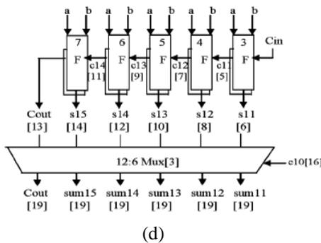
Fig.6. Delay and area evaluation of regular SQR CSLA:
