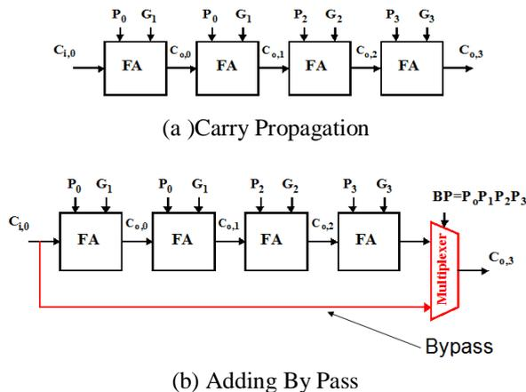
Fig.3. Carry skip adder structure – basic concept
