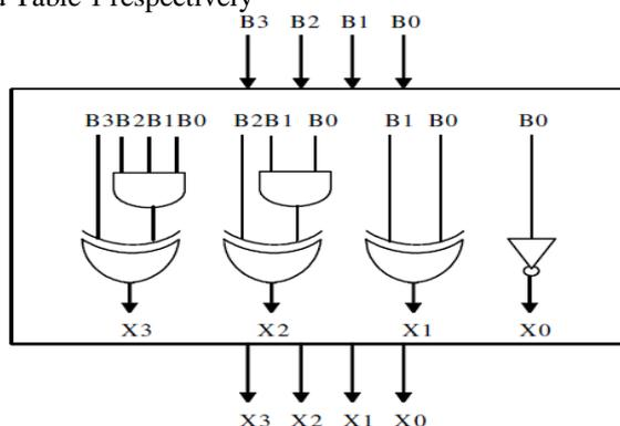
Fig.1. A 4-bit Binary to Excess-1 Converter (BEC)
