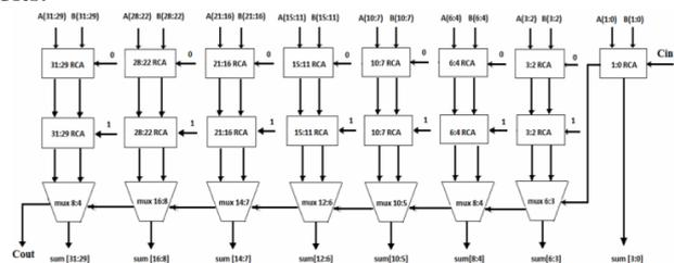
Fig. 5. 32 bit regular carry select adder
