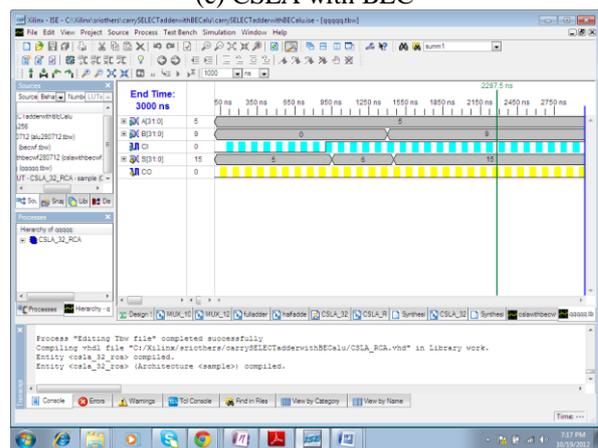
Fig.6: CSLA with BEC and RCA
