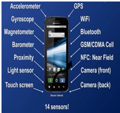
Fig: 1 Accelerometer Sensor X, Y, Z axis and all Sensors in Mobiles
