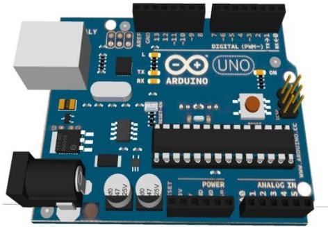
Fig.6. Arduino Uno Board
