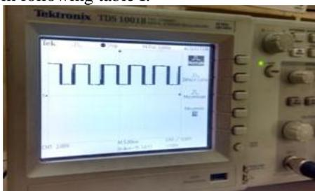
Fig.4. Heart rate sensor waveform
