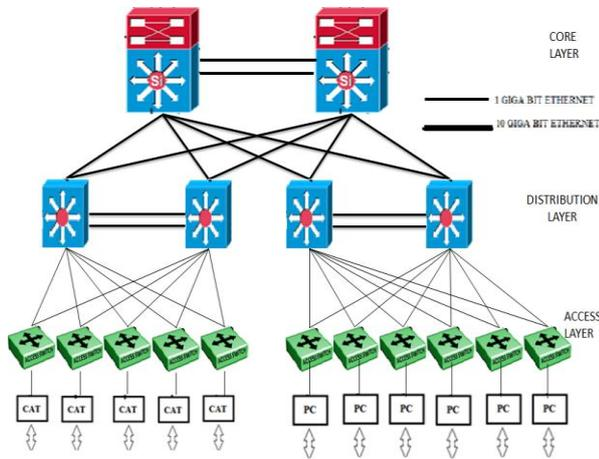
The Access layer having a myriad of Ethernet Edge Switches is the outermost layer and is intended to provide connectivity to the end equipment of all systems. The Distribution layer having two dedicated distribution switches for each system is positioned between the Core layer and the Access Layer providing connectivity between the two layers.
