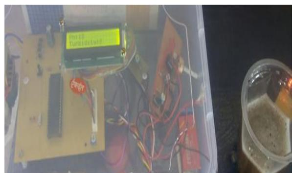
**Figure 11: Turbidity=8 indicate unsafe water**
