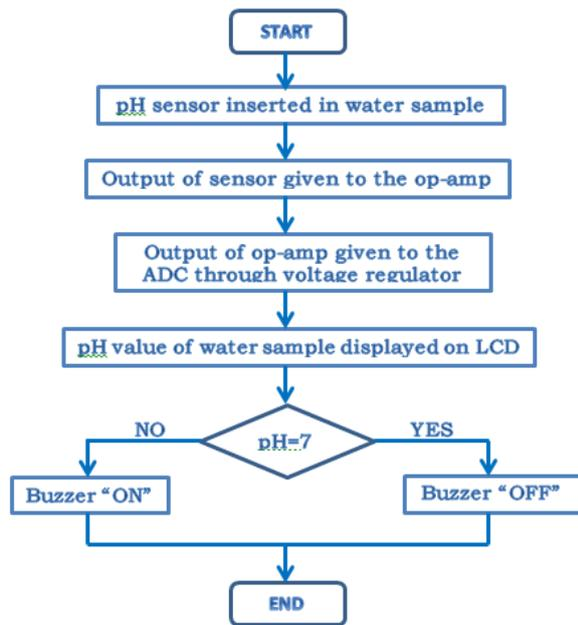
**Figure 6: Flow chart showing operation of pH sensor**
