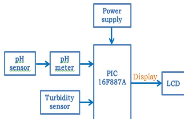
Figure 5: Block diagram of proposed system
