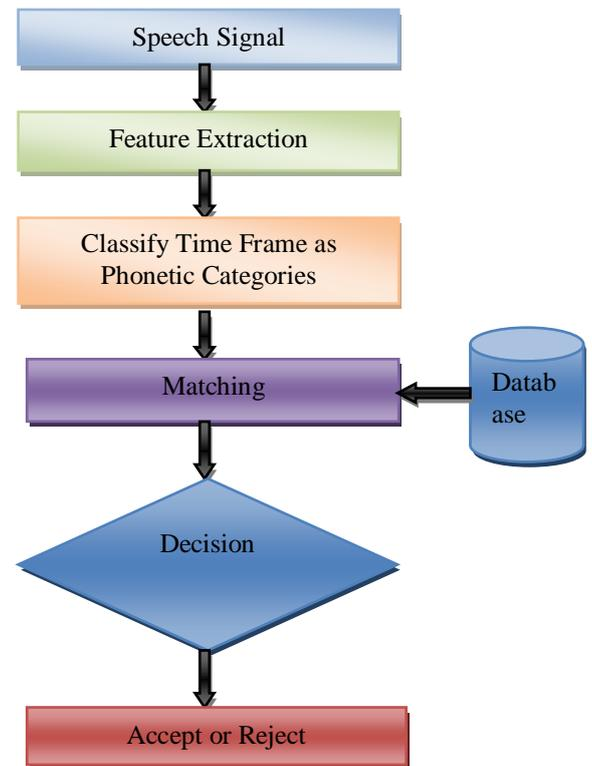
Fig.1: Flow Diagram of Speech Recognition System
