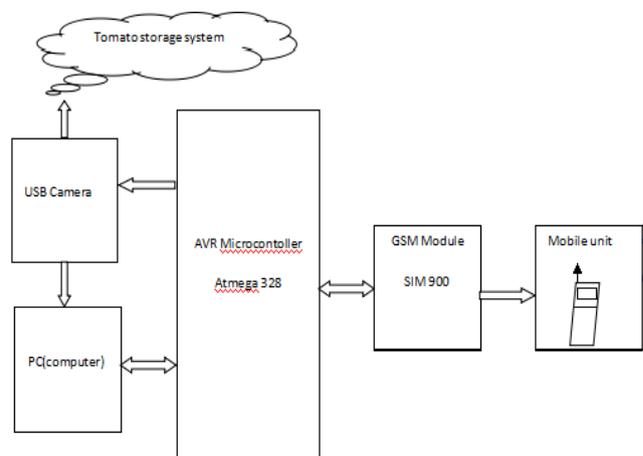
Figure 2: General Block Diagram of the system
