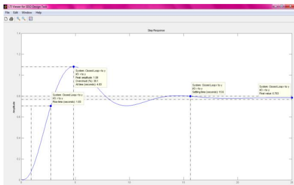
Fig (5)-pitch control system response for k=5
