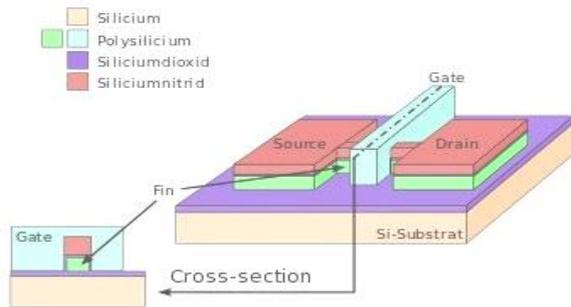
Fig: 2 Schematic diagram of FinFet
