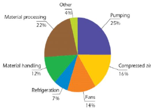
Fig.1.3 electric use by types of electrical motor.
