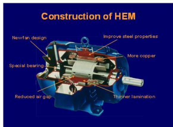
Standard motor is a compromise between efficiency, endurance, starting torque, and initial cost (with strong emphasis on the initial cost). Standard motor generally competes on price, not efficiency on the contrary. EEM competes on efficiency. not price.
