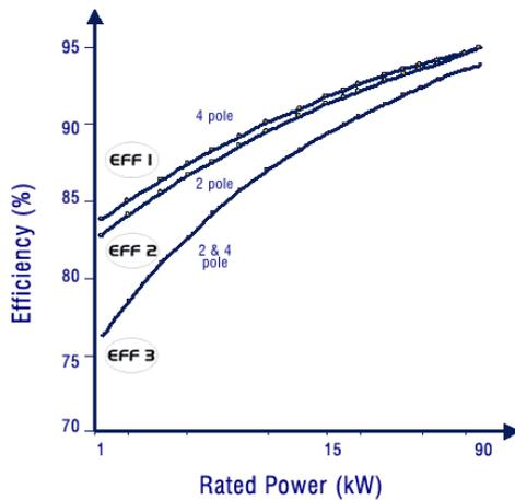
Fig 1.2 –Curves Efficiency –Rated Power
