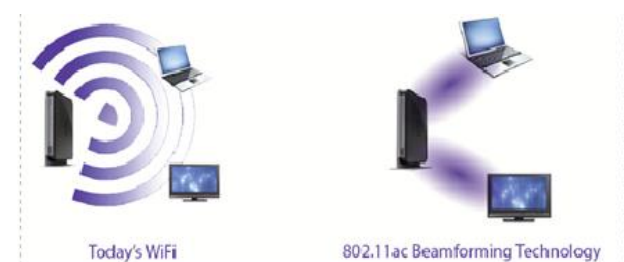
Figure (3): 802.11ac and 802.11n differences in connection approach and methodology
