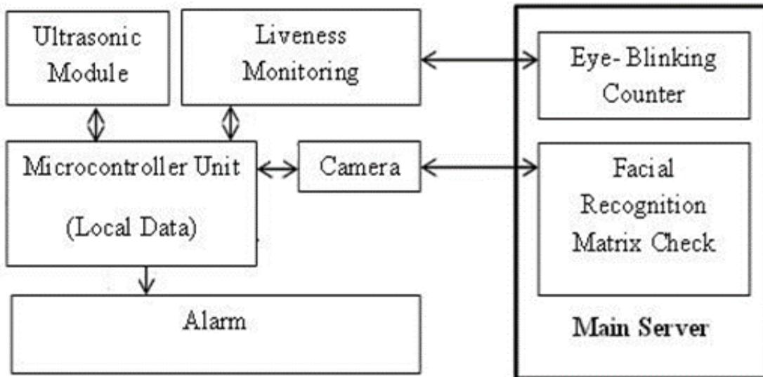
Figure No. 4 Block Diagram of Proposed System
