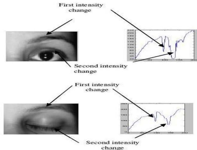
Figure No. 5 Eye Blinking identification process
