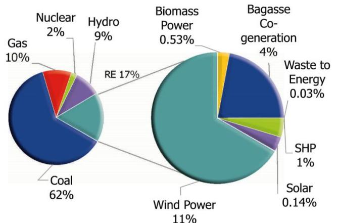
Fig.1: Resource wise installed capacity in Maharashtra
