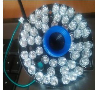
Fig 2b LED Ring with VGA camera
