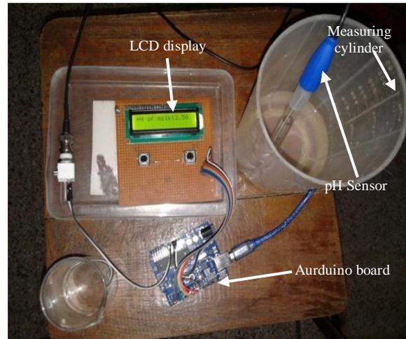
Fig.3: The pH measurement setup
