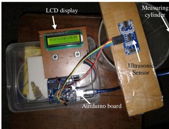
Fig.2: Milk quantity measurement setup
