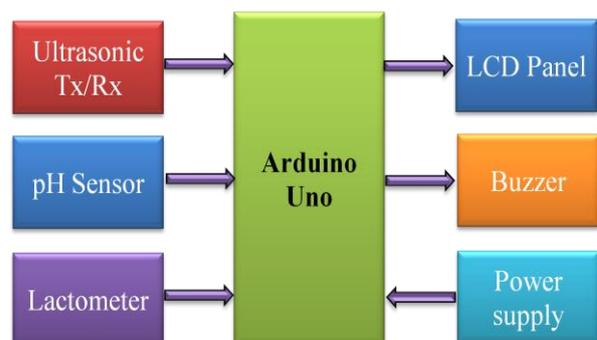
**Fig 1:** Block diagram of Milk parameter measurement system
