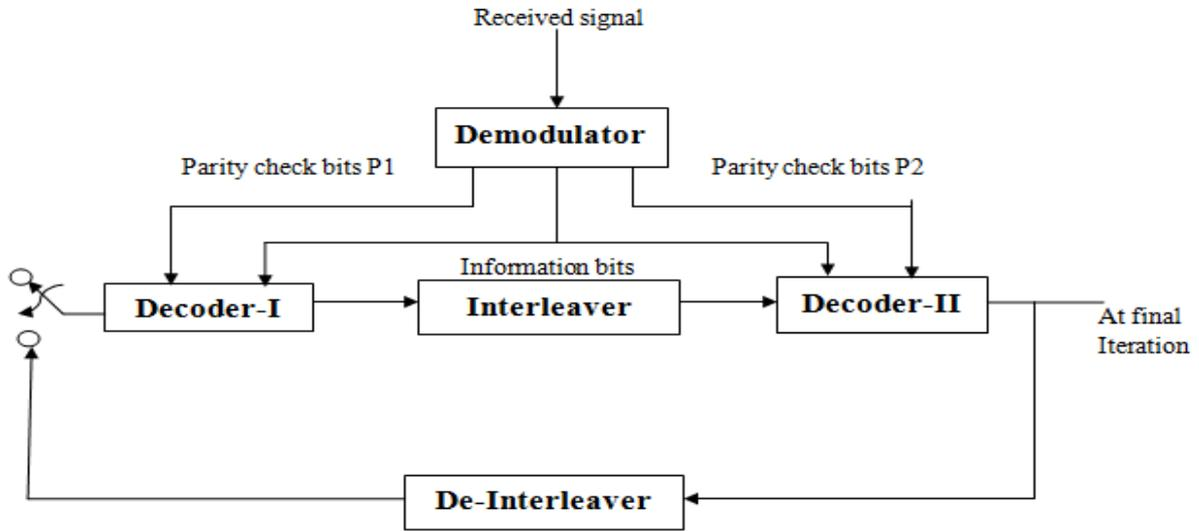
Figure 5: Turbo decoding
