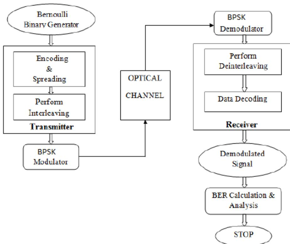
Figure 1: Transmitter and receiver configuration of turbo oidma system with k user.
