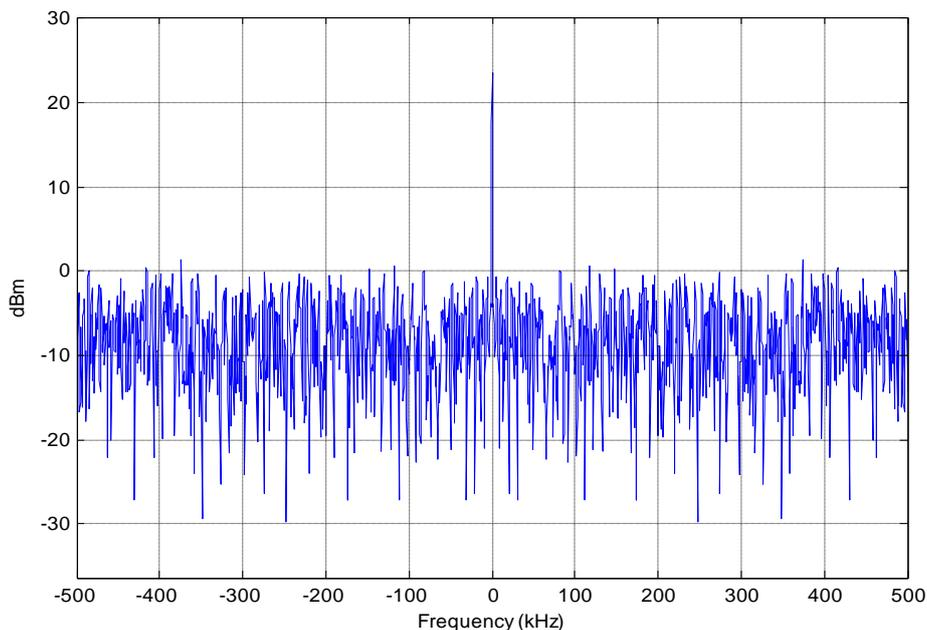
Fig6: Spectrum analyser output of oidma scheme with turbo encoder.
