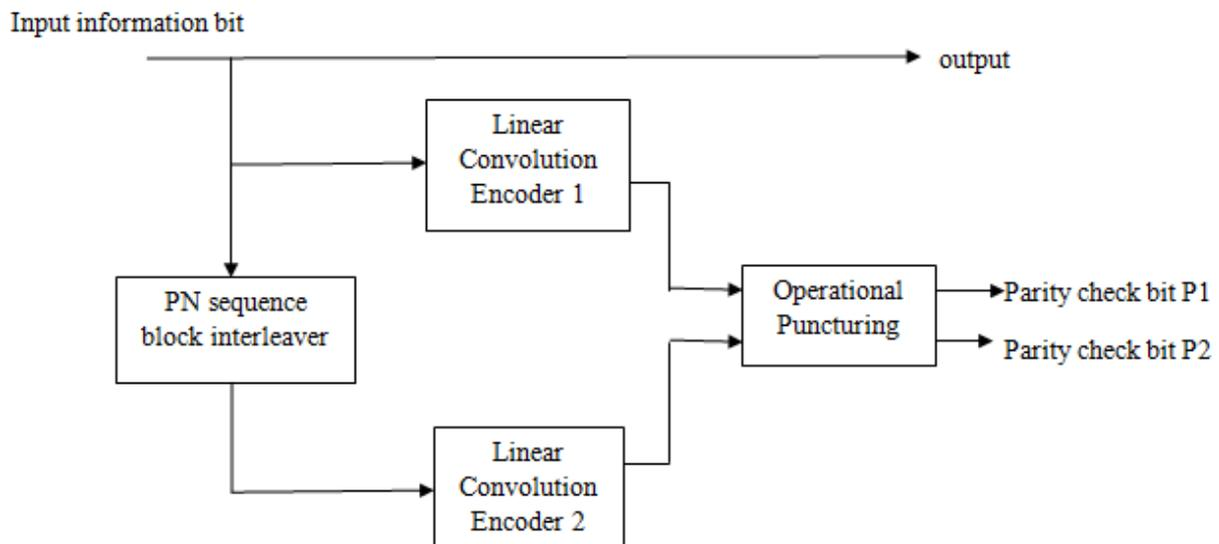
Figure 2: Internal structure of turbo encoder.
