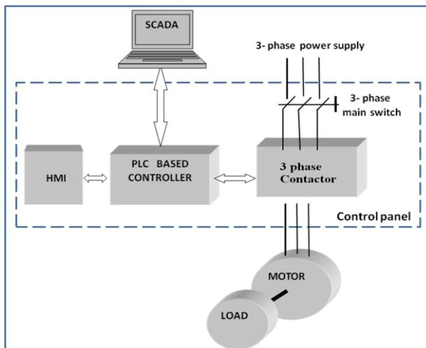
Fig. 1: Block diagram of SCADA system
