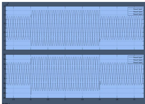
Figure 6: Effect of Swell on Voltage & Current
