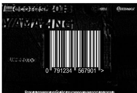
Fig.3 Image after applying gray thresholding
