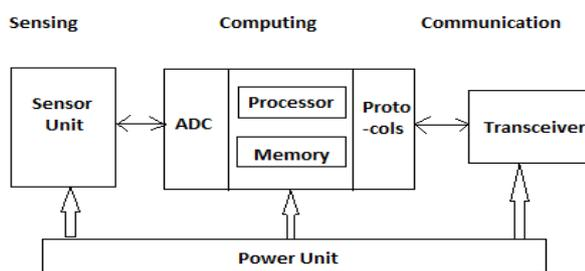
Figure 1: Components of Sensor Node
