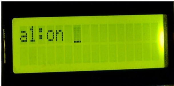
Fig.10. Receiver LCD status when device 1 in ON
