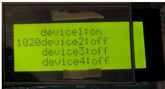
Fig.9. Transmitter LCD status when device 1 in ON
