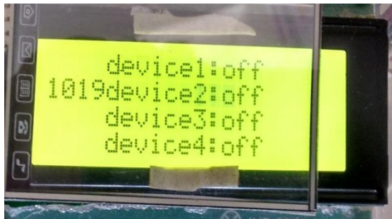
Fig.7. Controller LCD status when system is initialized
