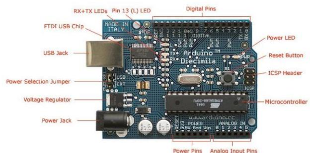
Fig. 1 Arduino embedded board with microcontroller
