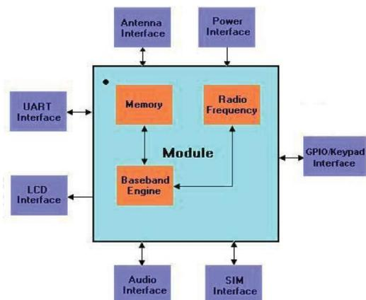
Figure 4. SIM900A functional diagram
