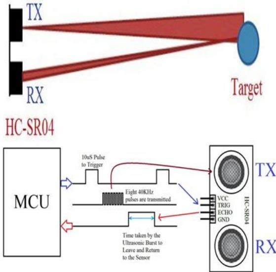
Figure 3. Working of ultrasonic sensor.
