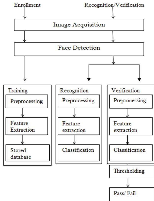
Figure 1: Block Diagram for the Proposed System
