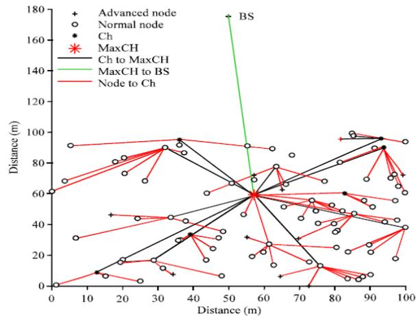
**Fig:4 Dynamic oriented cluster formation using OCFLE**
