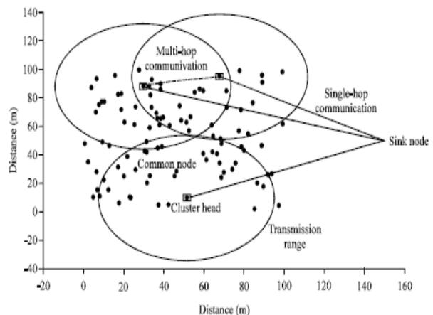
Fig.3: Architecture of a wireless sensor network
