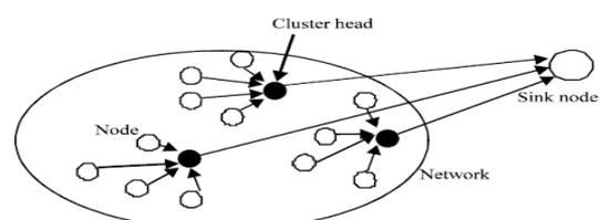
Fig.2: Example of Node Clustering in WSN
