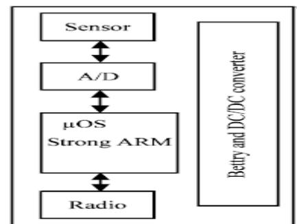
Fig.1:Sensor Node Architecture
