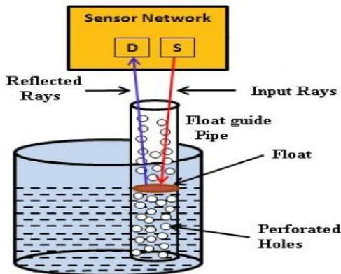
Figure 7 Optical Water Level Sensors
