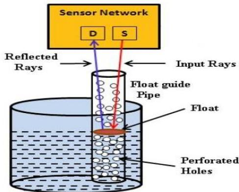
Figure 7 Optical Water Level Sensors
