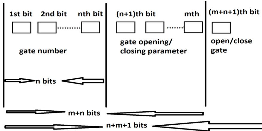
Figure 15 Decoded Signal
