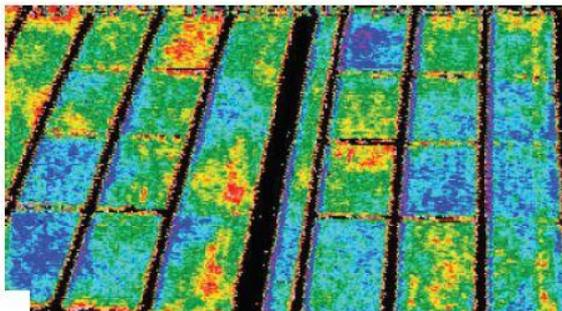
Water content of crop fields with thermal imaging. Blue, green and red pixels represent plants with sufficient, average and low water concentration.
