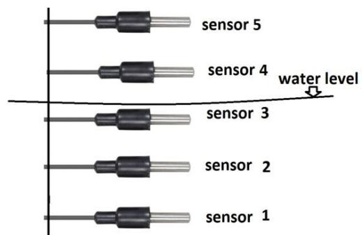
Figure 6 Array of water level sensors
