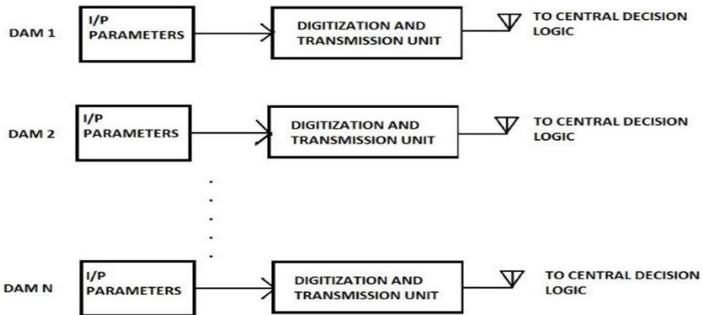
Figure 3 Monitoring and Transmission System
