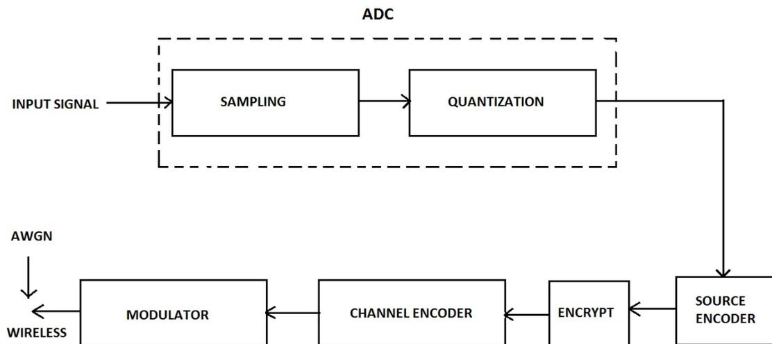
Figure 9 Block diagram of digitization and transmission unit
