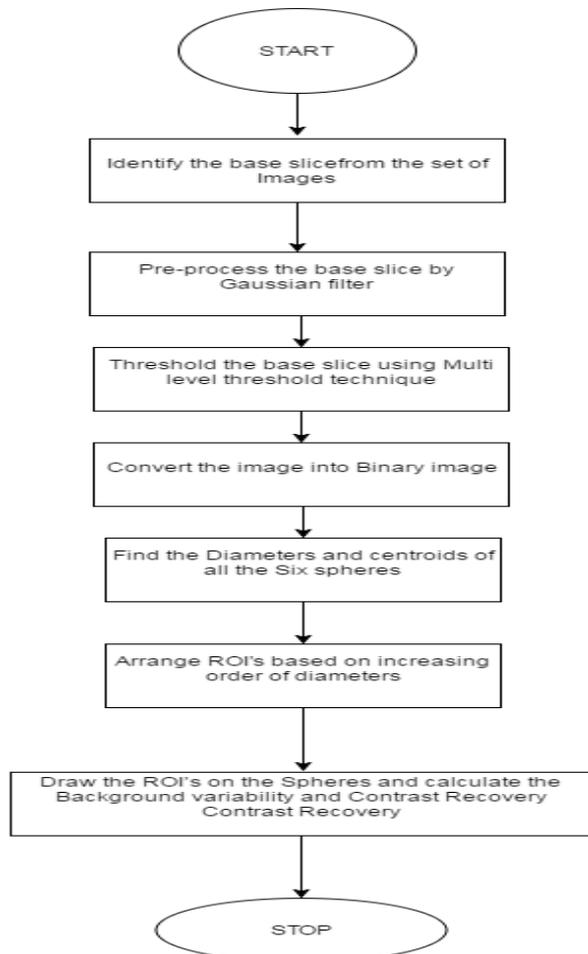
Fig 3: Flowchart for Automatic Placement Of ROI's in NEMA-IQ Tool
