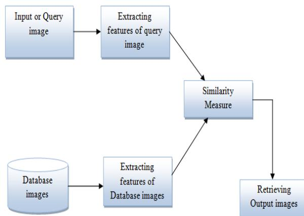
Fig. III.1 Architecture of CBIR system
