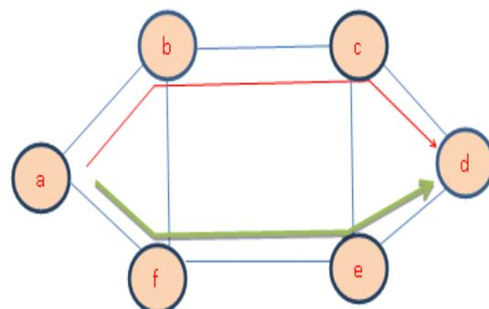
Figure 3: Fixed Alternate Routing from node a to d.
