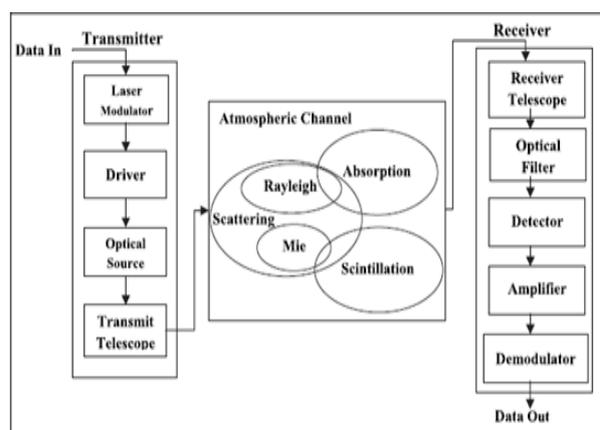
Figure 1: Block Diagram of FSO System
