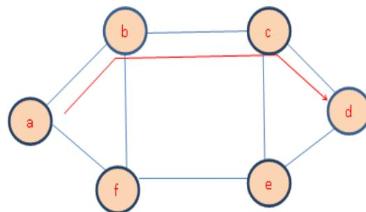
Figure 2: Fixed Routing from node a to d.
