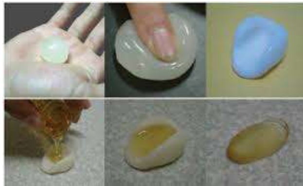
Fig 1.1 : Making an artificial fingerprint directly from live finger plastic , used to obtain the mold and gelatin to obtain the cast.
