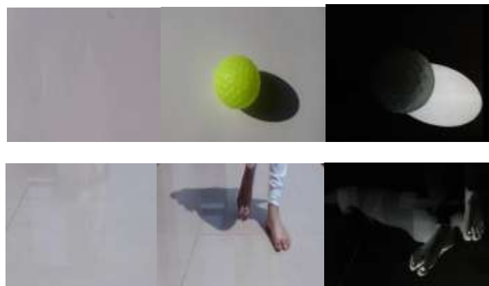
Fig 2. Results of the Flowchart a) Reference image b) Foreground image c) Subtracted image
