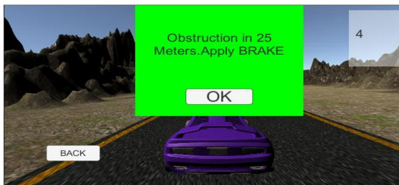
Fig. 4 Low level Prompter appears at a distance of 25 meters from static object
