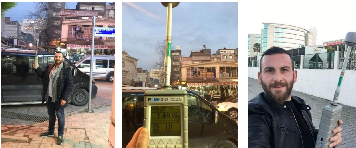
Fig. 3 EMR measurements with PMM-8053
