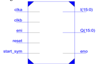
Fig.12 RTL View of Pilot Generator
