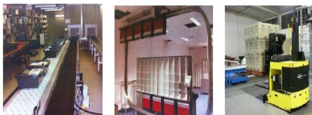
Fig. 2.2 Rail system, Pneumatic Tube System and Automated Guided Vehicle
