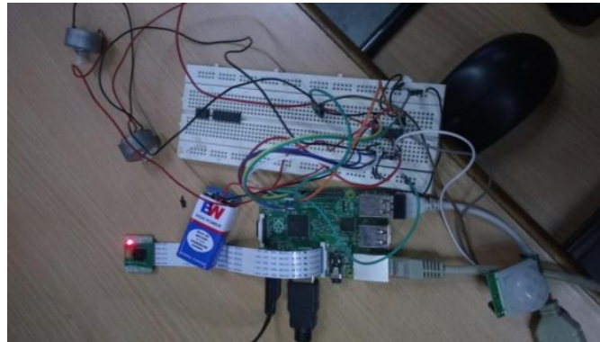
Fig.6.1 Testing of Motor Driver
