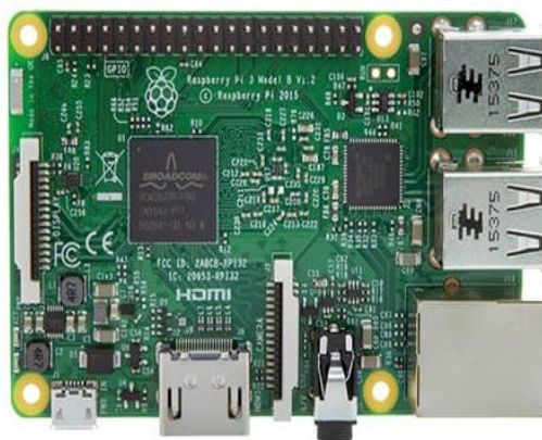
Fig. 4.1 Raspberry Pi Board Type-3
