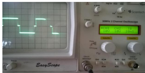
Figure:8 Clipping of square wave in hardware
