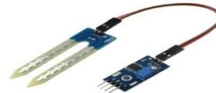
Fig; Soil moisture sensor
