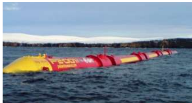
Fig.1: Actual view of Snake Wave energy installation
