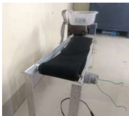
Figure: 10. Conveyor belt assembly
