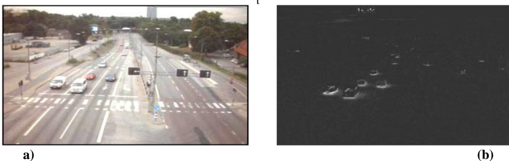
Fig 3: (a) Real-time image extracted from the live video (b) Difference of reference and real time image
