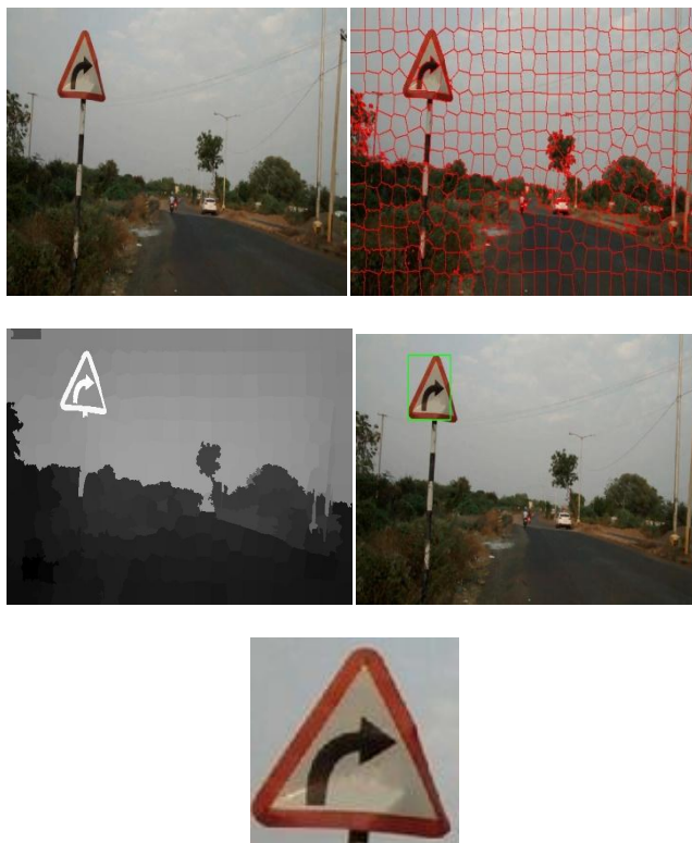
Fig.3.1 First row images, Input image (left) and segmented image (right). Second row, saliency image (left) and Region of Interest (right). Last row represents the salient object being isolated.
